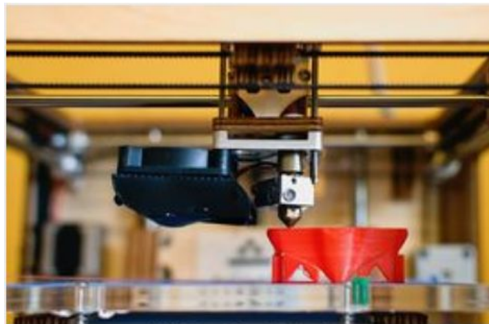
Image 2 – 3D printing of a polymeric part.
