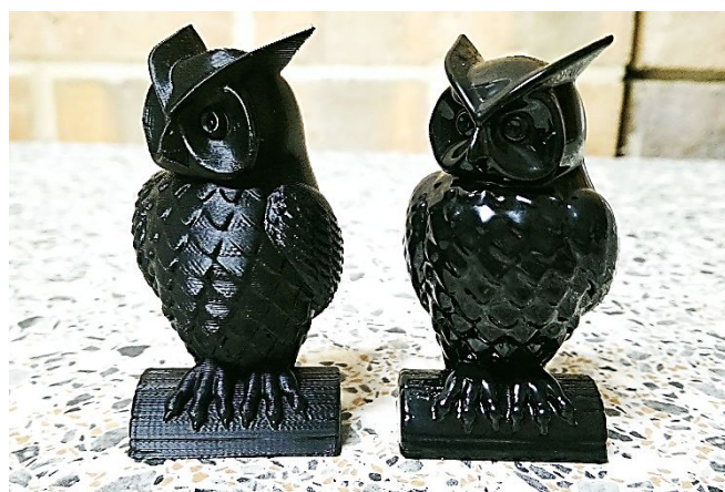
Image 3 – 3D printed object before and after being post-processed.
